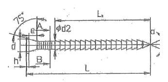
Special nail NFX-Norfix or an equivalent nail
